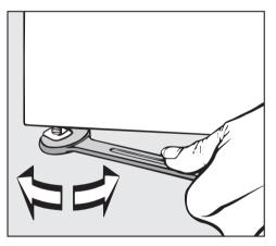
The screw feet can be adjusted to compensate for any unevenness in the floor. The air inlet and outlet vents on the front and back of the machine must not be covered as this would prevent sufficient ventilation for cooling the condenser unit.
